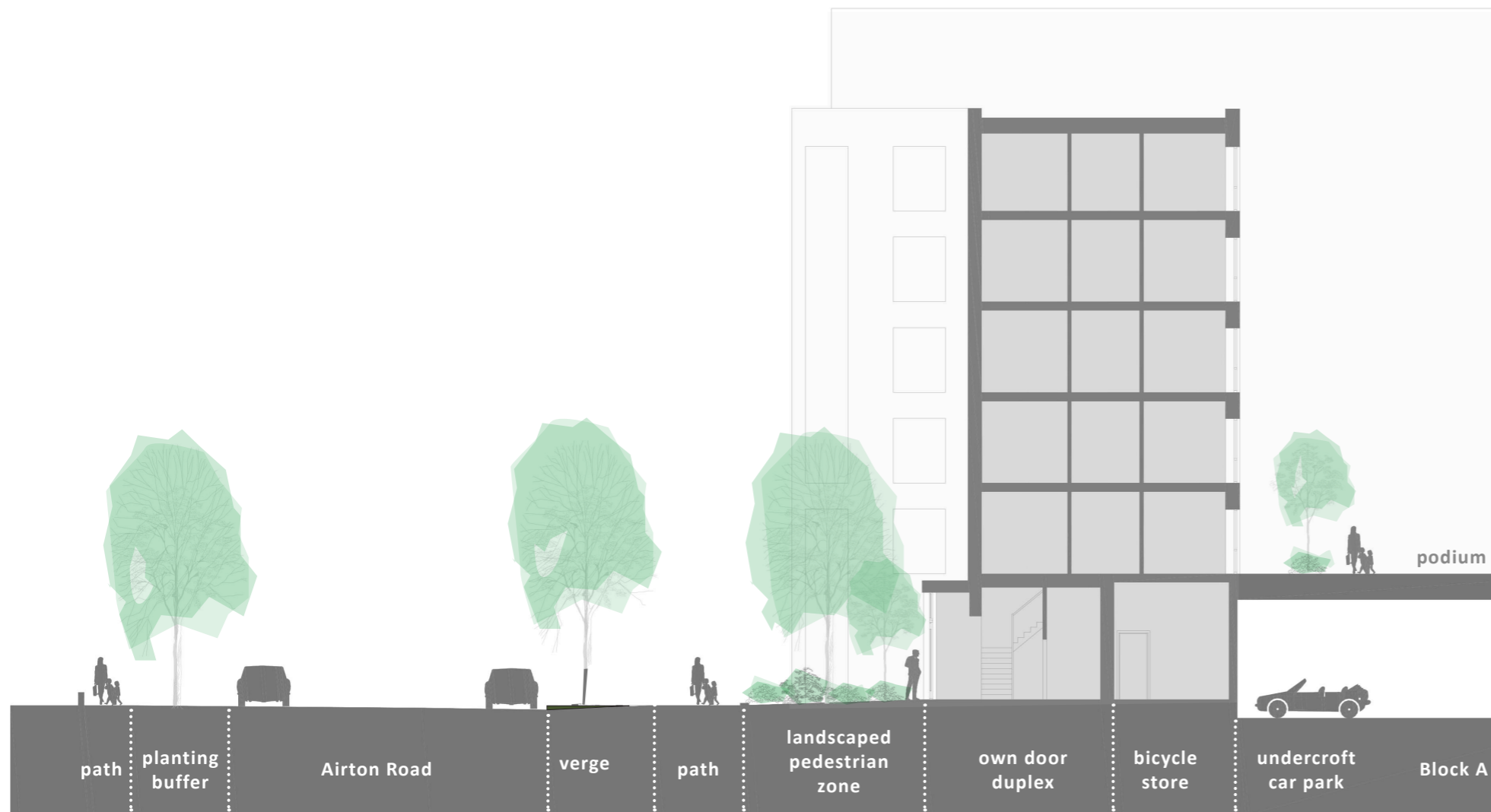
Section showing Airton Road
